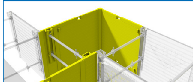
Closing off a 90° bend in the course of the trench (district heating lines)
