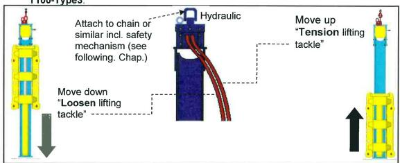
Test whether the working function of the attachment can be controlled by the hydraulic controls in the carrier, as described in the carrier's operating instructions:
