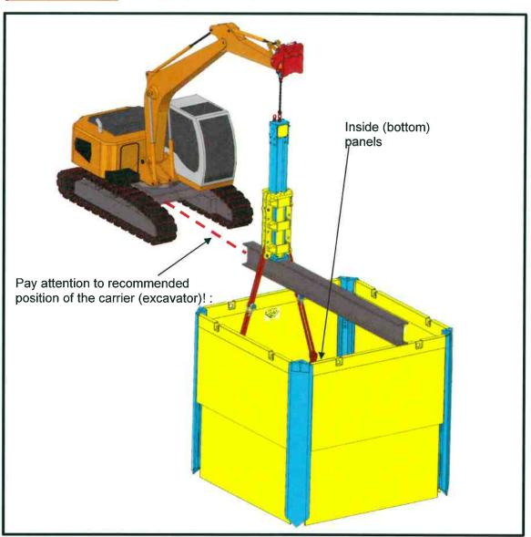
In some circumstances there is no need to use a carrier and the **Hydralifter T100-Type3** can be directly placed onto the outer panel.
